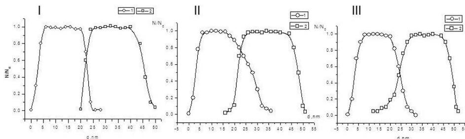
**Figure 7.** Distribution of atoms in the two-layer Ni-Fe film: 1-Ni, 2-Fe; I - non-irradiated film, II - the film irradiated by the excimer laser pulse with the energy density  $W=0.6$  J/cm<sup>2</sup> from the nickel layer, III - the film irradiated by the excimer laser pulse with the energy density  $W=0.6$  J/cm<sup>2</sup> from the iron layer.
