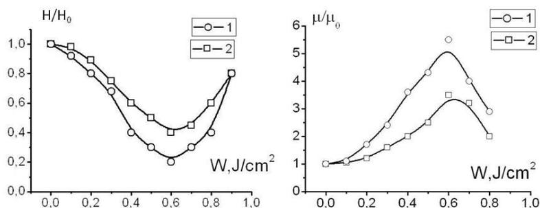
**Figure 5.** Relative change of magnetic permeability  $\mu$  and coercive forces  $H_c$  in film  $Ni_{81}Fe_{19}$  with thickness 250 nm (1) and 500 nm after irradiation one pulse of excimer laser with density of energy  $W=0,6$  J/cm<sup>2</sup>.
