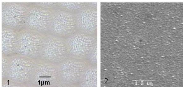
**Figure 2.** Photos of the film surface after irradiation pulses of Nd:YAG laser ( $\lambda=355$  nm): 1 – the sequence of single pulses, the laser beam diameter is 3-5 microns; 2 – the result of destruction of the film, the diameter of the laser beam was less than 1 micron.
