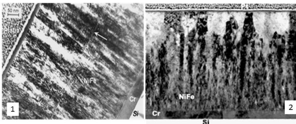
**Figure 6.** Change of crystal structure of  $\text{Ni}_{81}\text{Fe}_{19}$  film with a thickness of 500 nm after an irradiation one nanosecond pulse of excimer laser with density of energy  $W=0,6$  J/cm<sup>2</sup>: structure of cross-section section of the film to irradiation (1); structure of cross-section section of the film after irradiation excimer laser pulse with the density of energy  $W=0,6$  J/cm<sup>2</sup> (2).
