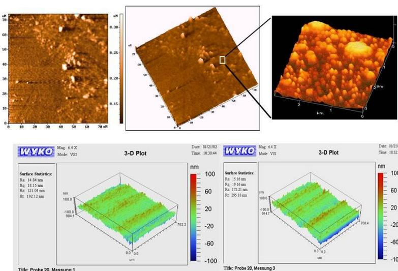
**Figure1.** Change in the roughness of surface of  $\text{Ni}_{81}\text{Fe}_{19}$  film after irradiation with one pulse Nd-YAG laser (top, spherical lens) and excimer laser (bottom sequence of three pulses focused by a cylindrical lens).
