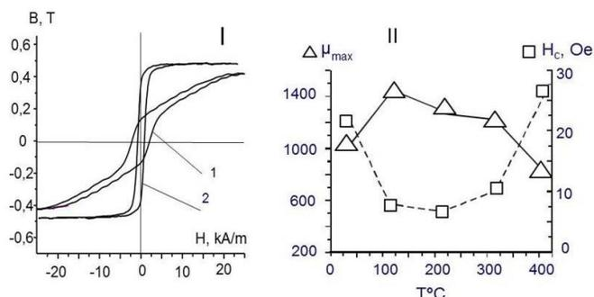
**Figure 4.** Change of the form of the switching curve (I), and also magnetic permeability  $\mu$  and coercive force  $H_c$  (II) in film  $Ni_{81}Fe_{19}$  with the thickness of 500 nm after an irradiation single nanosecond laser pulse: I-1 –switching curve loop of magnetic reversal to an irradiation, I-2 –pulse of Nd:YAG laser ( $\lambda=355$  nm  $W=0,6$  J/cm<sup>2</sup>), II-2 – pulse of excimer laser ( $W=0,6$  J/cm<sup>2</sup>) at various reference temperature of the film.
